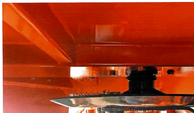
The large distance between the knife and the frame construction ensures smooth work with the best shredding quality.
