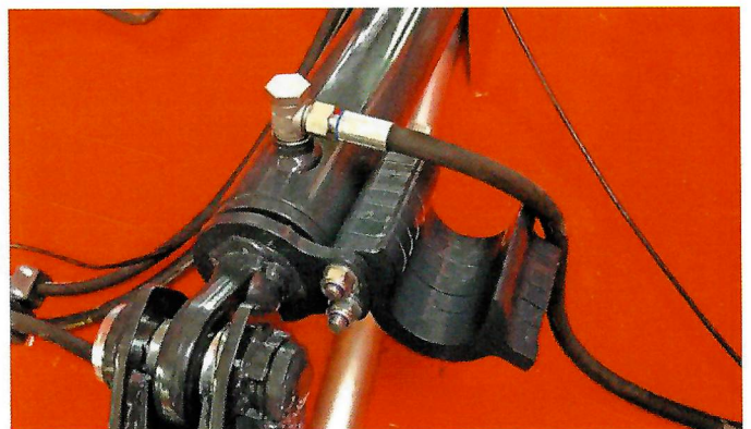
The height is adjusted using 3 hydraulic cylinders, each of which has attached segments.
