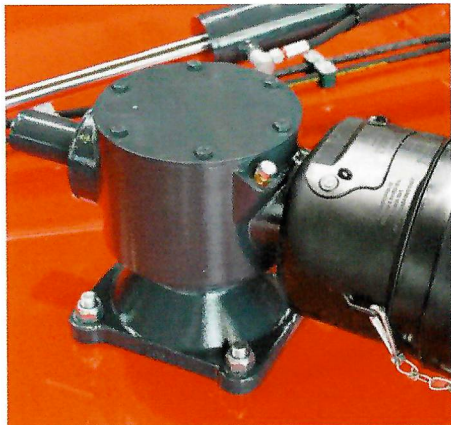
Rotor gearbox - with ventilation 180 hp max. power - oil volume: 3.5 liters.
