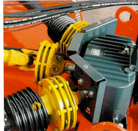
PTO shaft with 2-disc slip clutches.
