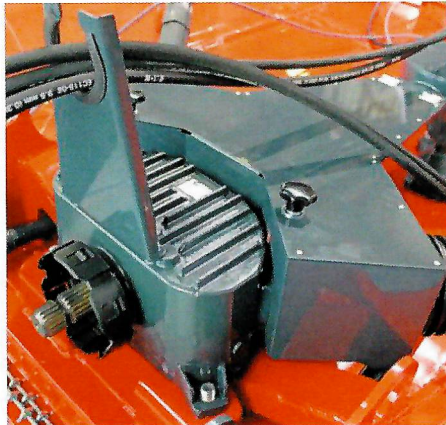
Splitter gearbox - with ventilation 290 hp max. power - oil volume: 3.8 liters.
